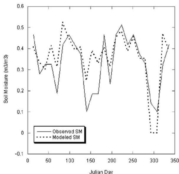
**Figure 6.** Observed and ‘modeled’ soil moisture at Fletcher, NC. The observations were taken continuously at a depth of 10 cm (every hour and then averaged to a day). The ‘modeled’ value is estimated as 75% of the SPI (normalized as discussed in the text), multiplied by the saturation limit of the soil (taken as  $0.7 \text{ m}^3 \text{ m}^{-3}$  for this site).
